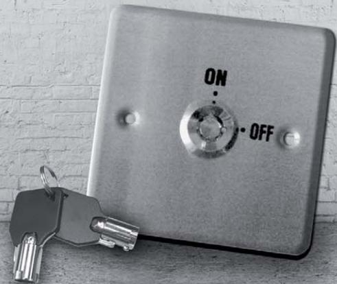
The Override Key Switch is designed to be installed in a secure location outside, wired in parallel or series with the power supply and the electromagnetic lock (EM lock). If the EM lock malfunctions due to the failure of the reader or other reasons, the user can switch between normally closed (N.C.) and normally open (N.O.) contacts by using the key, thus forcing the door to open. Override Key Switch is used as a backup to an access control system.
