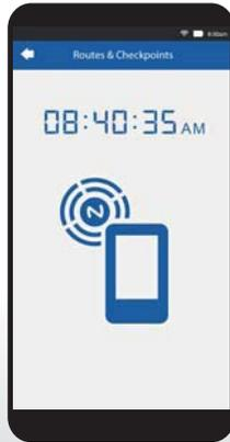
NFC tags are installed at regular intervals at each patrol route for monitoring purpose. Each guard is assigned with an NFC-enabled phone during his patrol rounds. When the guard places the phone near any tags, a signal is sent to TimeTec Patrol's cloud portal along with information regarding the identity, time, and exact location of the guard.
