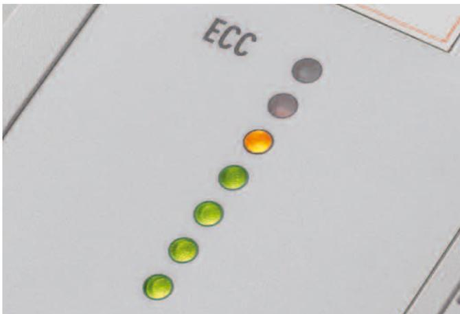
**ECC – ELECTRONIC CAPACITY CONTROL** ECC – Electronic Capacity Control indicates the used sheet capacity during shredding process to avoid paper jams.
