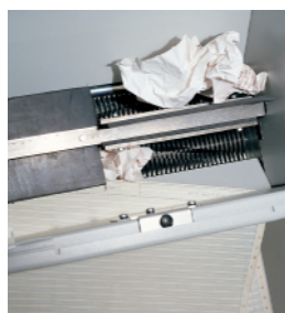
Automatic mechanical feeding system with revolving flaps
